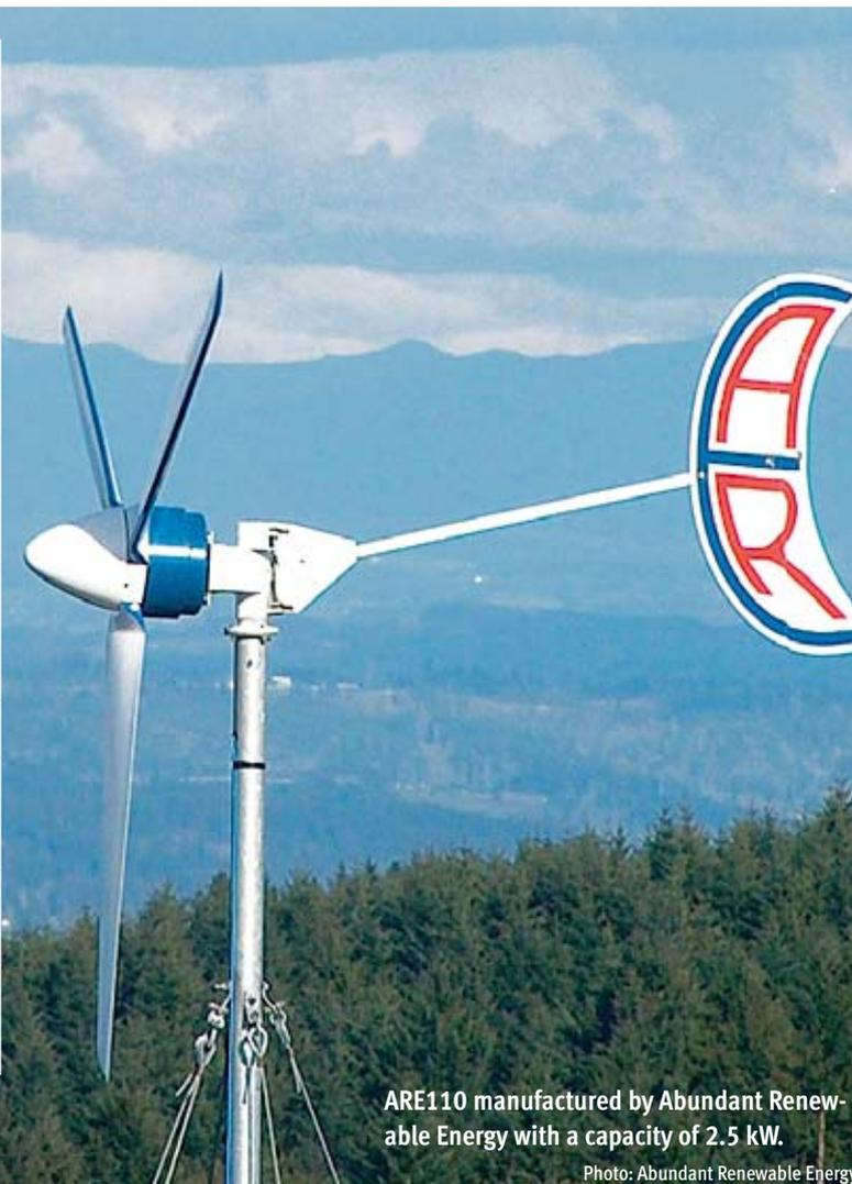
ARE110 manufactured by Abundant Renewable Energy with a capacity of 2.5 kW.
